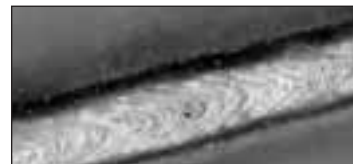
Power Mode aids bead wetting and penetration on aluminum.
