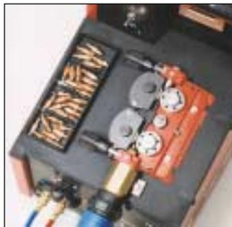
are equipped with the same rugged four-roll drive system. This drive is easy to access and protected by the unique flip-top cover. The wire guidance from the coil to gun tip is smooth and accurate. It is designed to eliminate tangles and guarantee trouble free feeding.
